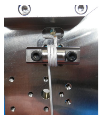
(c) Clamping with cylindrical block (D 15 mm × W 45 mm)
